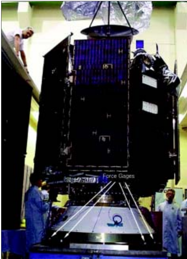
Figure 12. QuikSCAT combined vibration test.
