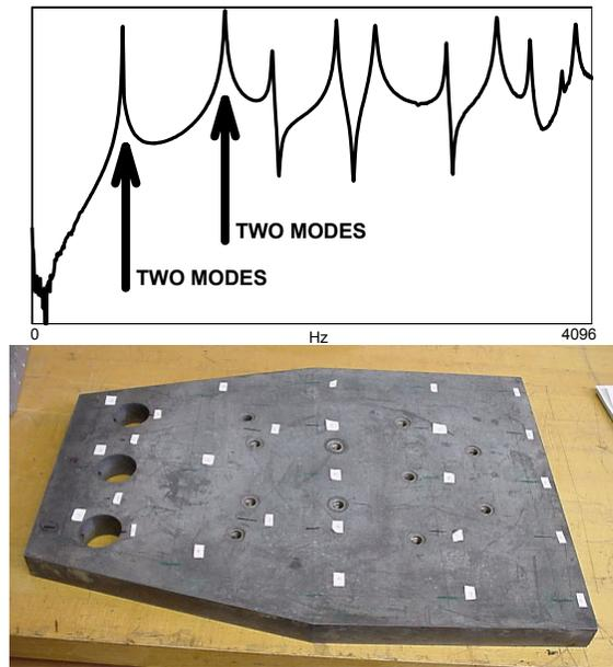
Figure 3 - Typical FRF and Photo of Structure
