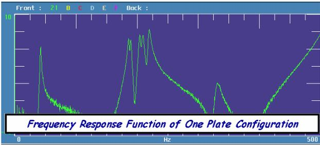
Figure 2 – Typical FRF Measured on Composite Plate
