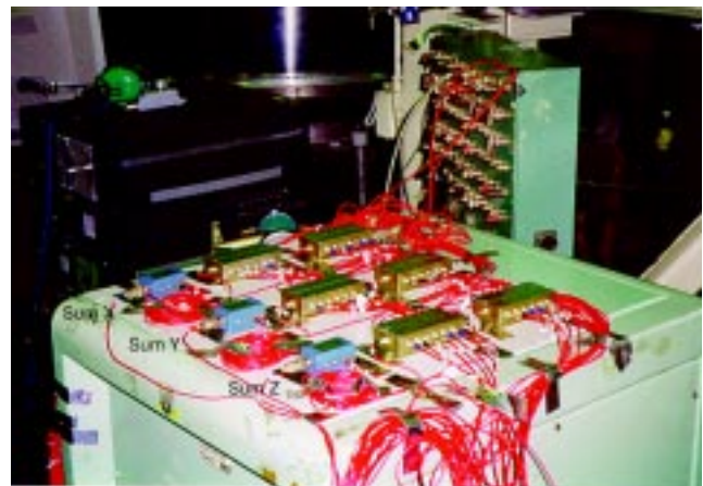
Figure 7. Summing of 24 force measurements in X, Y and Z directions.
