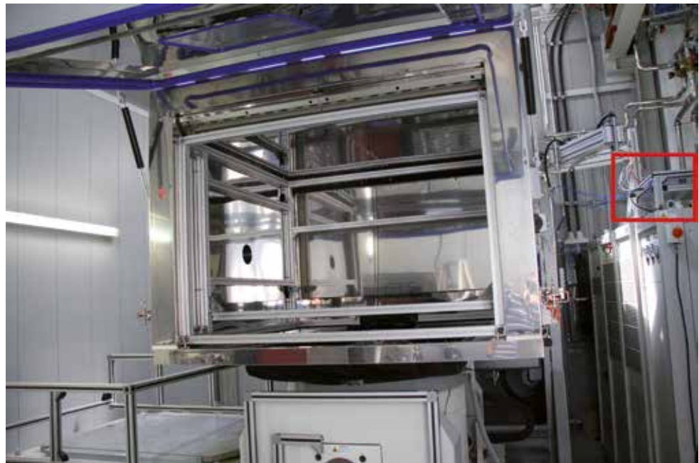
ABOVE: Vibration test rig with M+P International measurement front end
