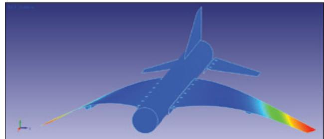
Figure 10. First flexible-body mode shape.
