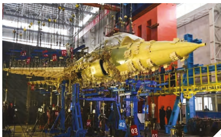
1 // China's Aircraft Strength Research Institute provides ground testing for full-size aircraft
