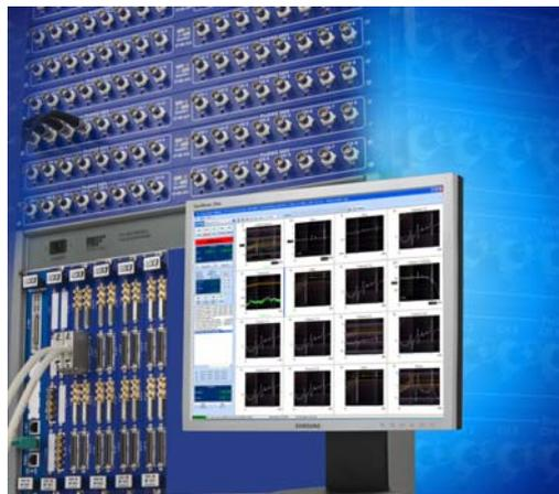
For continuous time domain recording the data is directly stored on two 250 GB hard disks. VibExec records this data at a constant bandwidth which is equal to or higher than the control frequency range. By using the hard disks in a parallel way, there are higher transfer rates possible than those of the single drives - and even with a higher security.
