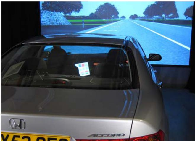
The project used SVT's Full Vehicle NVH Simulator which is based around a typical family saloon as shown on the left. The vehicle is driven exactly as it would be driven on the road because the stimuli are driver-in-loop. This means that the noise, vibration, visuals and steering feel all respond in real-time to:
