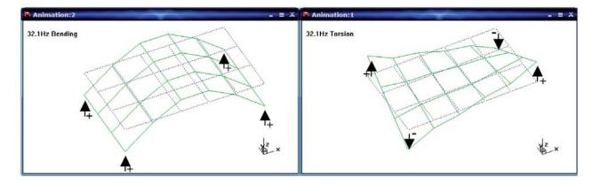
In reality the measurement is made whilst the frequency is swept or stepped through the resonance so that least squares methods can be used to improve the estimation of the modal parameters. The stepped technique is more rigorous than sweeping as it allows settling of the structure and then averaging of the data.
