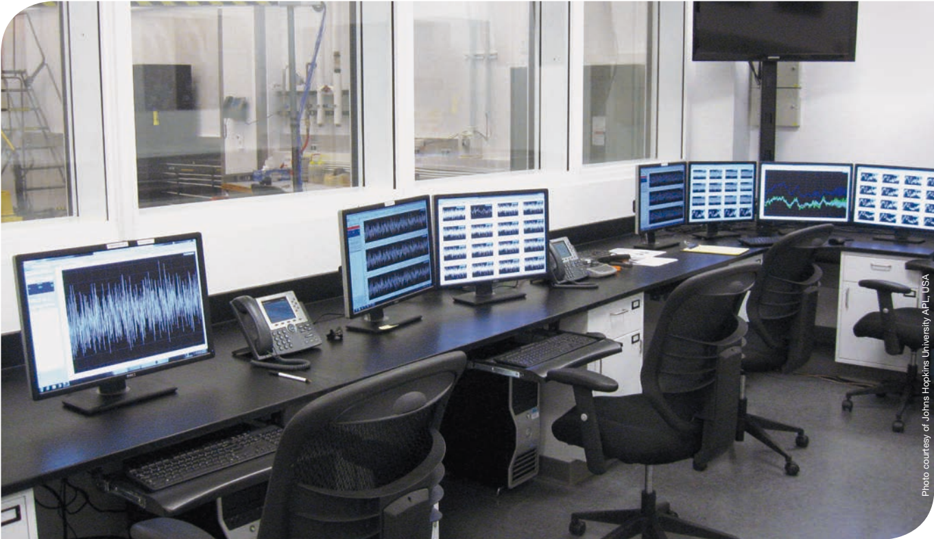
High-channel count data acquisition and vibration control system for large-scale spacecraft testing
