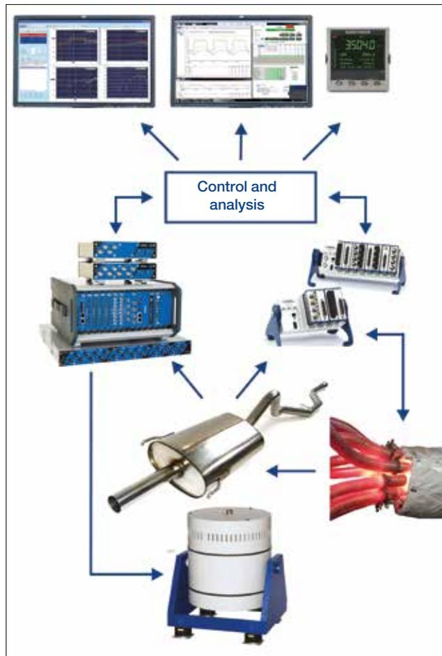
temperature and flow profiles and to guarantee that the specifications are followed. Additionally, a multitude of data channels, including thermocouples, pressure, voltages or digital conditions, are captured and monitored continuously using National Instruments hardware. This ensures that the correct skin temperature or average temperature of selected
