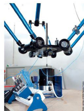
Modal analysis on a parallel robot
