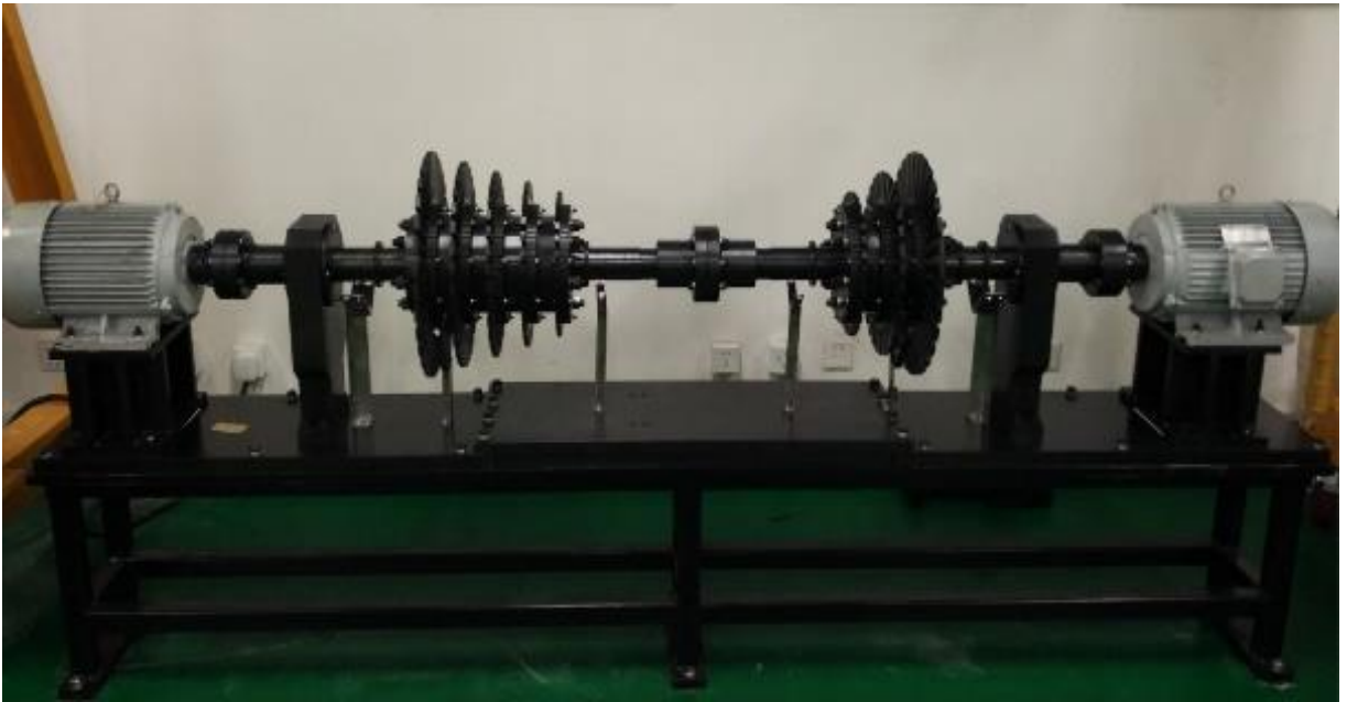
Figure 2. The structure of rod-fastening rotor
