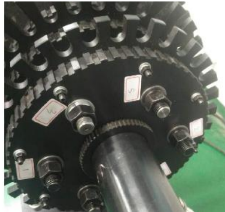
Figure 4. Pre-tightening sequence of the pull rods
