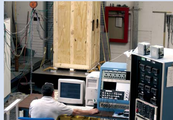
Earthquake simulation at Lucent Technologies, Whippany/New Jersey
