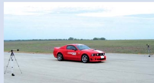
Pass-by-noise testing at Cooper Tire, USA
