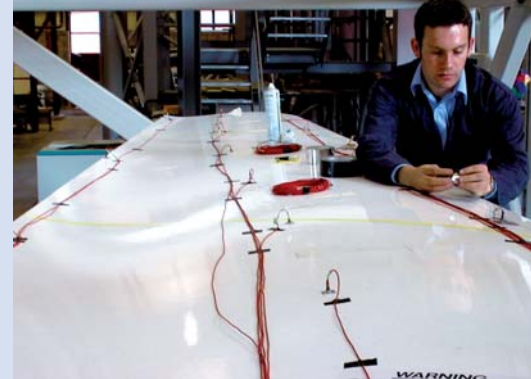
Testing A340 winglets at Stirling Dynamics, UK
